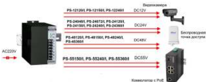
Рис. 5 Подключения блоков питания PS-12120/I, PS-12150/I, PS-12240/I, PS-24048/I, PS-24072/I, PS-24120/I, PS-24150/I, PS-24240/I, PS-24360/I, PS-48120/I, PS-48150/I, PS-48240/I, PS-48360/I, PS-55150/I, PS-55240/I, PS-55360/I
